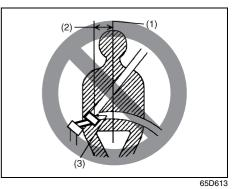
(1) Center of body(2) Less than 152 mm (6 inches)(3) Open end of extender buckle
